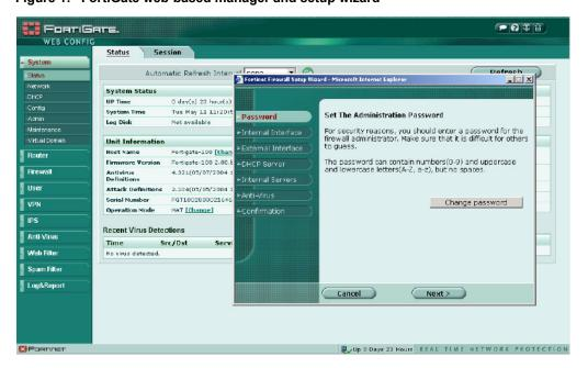
Figure 1: FortiGate web-based manager and setup wizard
